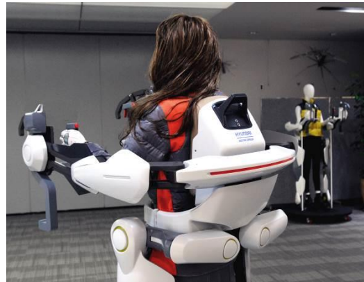
Fig. 36. Warning light on the back and sides
