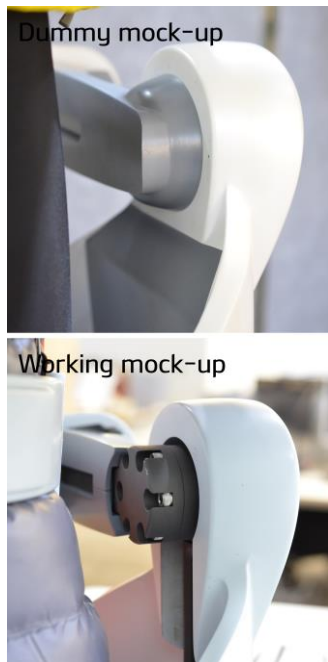
waist joints of dummy mock-up and working mock-up
